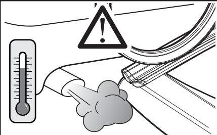
EN) Warning: Install the bike rack at a safe distance from the vehicle's exhaust pipe. The high temperature of the exhaust gases may damage the plastic parts of the bicycle rack.
