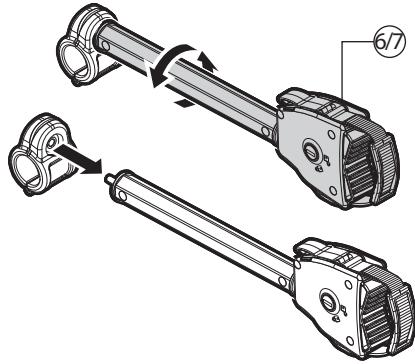
EN) Place the sealing ring on the "U" shaped pipe. Screw the frame holding arm to the frame-holder clamp with a torque of 2 Nm / 1.5lbf·ft.
