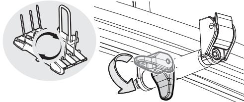
EN) Loosen the strap-lock lever.
