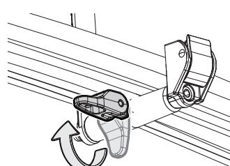
EN) Tighten the strap-lock lever.
