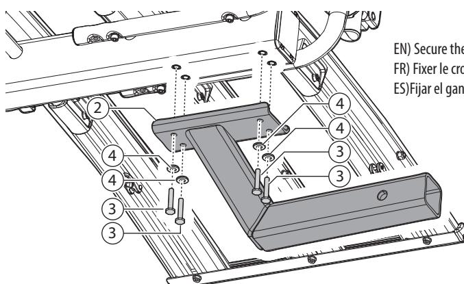
EN) Secure the hook to the bike rack using the screws and washers supplied.
