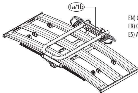
EN) Open the locking levers to loosen the hinge.
